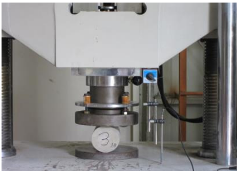
Fig. 8. Split tensile strength test
