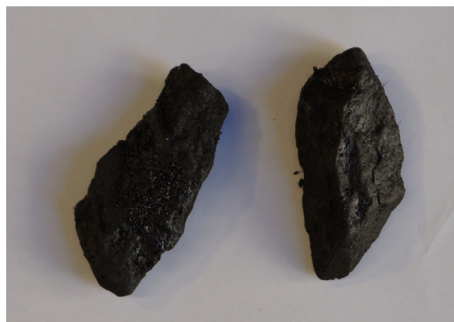
Fig. 2. Railroad ballasts contaminated with lubricant oils.
