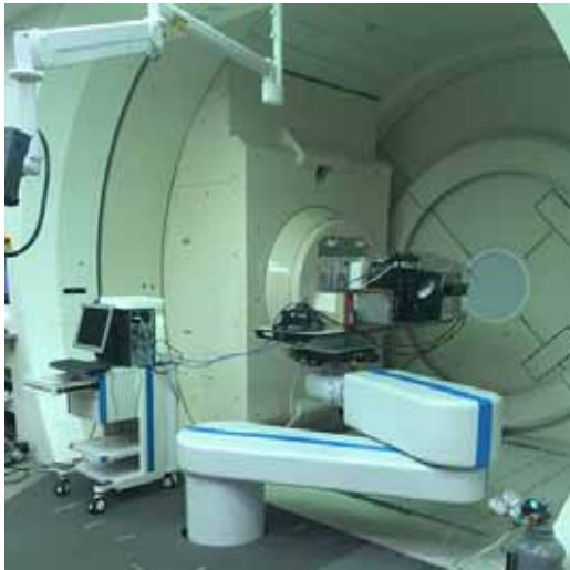
Fig. 3. Detector installed at a distance of 10 cm from the rectangular copper collimator, mounted in the rotating beam gantry, where a compensation Bolus, required to further focus the dose to the patient’s tumor, is to be placed.
