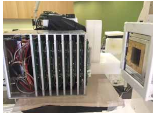
Fig. 1. Gaseous detector constructed with eight-layer interlaced thin PPICs and absorbers made of PMMA plates.
