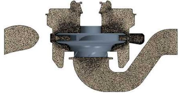
Fig. 2 Computational domain of centrifugal pump
