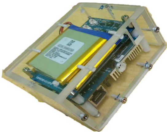
Fig. 5 ODROID board in case of a therapeutic doll
