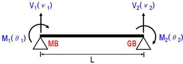
Fig. 4 Beam-Spring model for drive train
