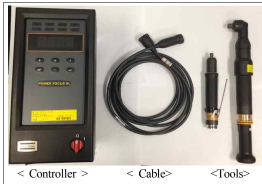
Fig. 3 Composition of power assembly tool
