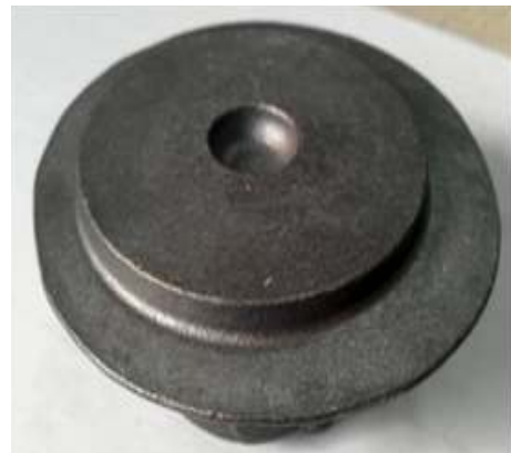
Fig. 16 1st hot forging product of Clutch Jaw after cooling
