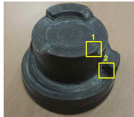
Fig. 21 Flatness measurement of Clutch Jaw product
