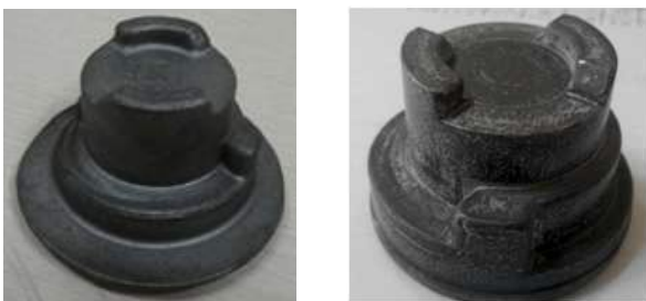
(a) 1st hot forging product (b) 3rd cold heading product
