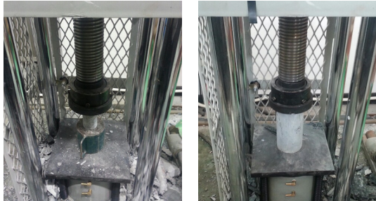
Fig. 10 Drilled core samples with different diameters and test setting for compressive strength
