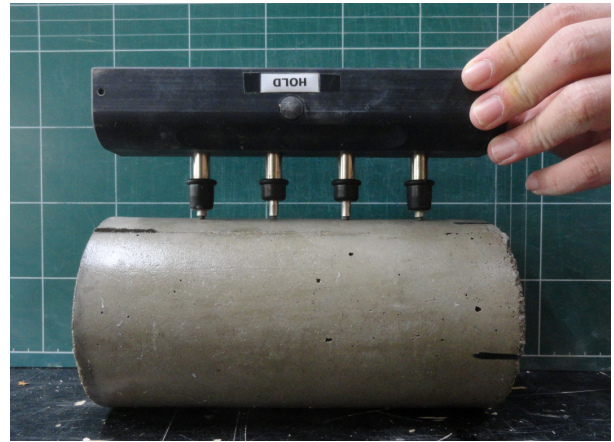
Fig. 3 Surface electric resistivity measurement
