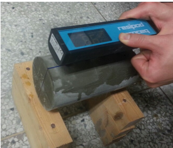
Fig. 12 Surface Electrical Resistance Measure
