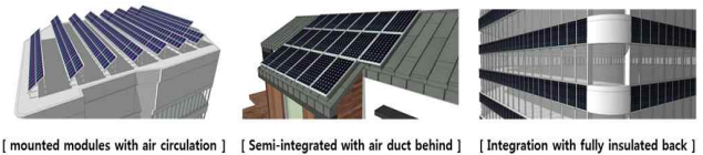
Fig 3. Installation types of PV systems
