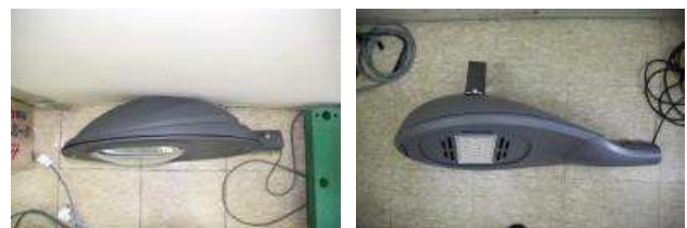
Figure 2. Luminaires with NH 100W, MH 70W(left), and LED 50W(right)
