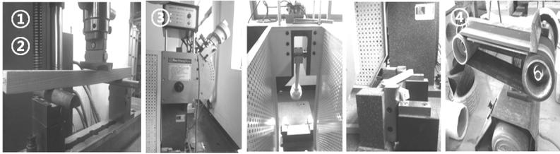
Fig. 2. Testing Machine (Bending, Fatigue, Impact, abrasion resistance).
