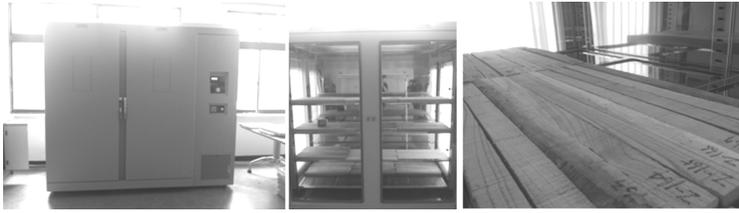
Fig. 1. Machine for Accelerated Weathering Test.
