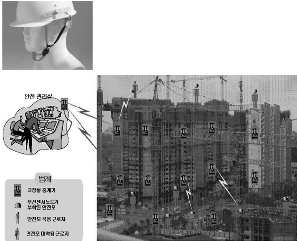
Fig. 1. Configuration of remote confirmation system for worker's helmet remove or not.
