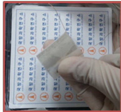
Fig. 6. Flexible piezoelectric NCG device based on BaTiO 3 dendrite
