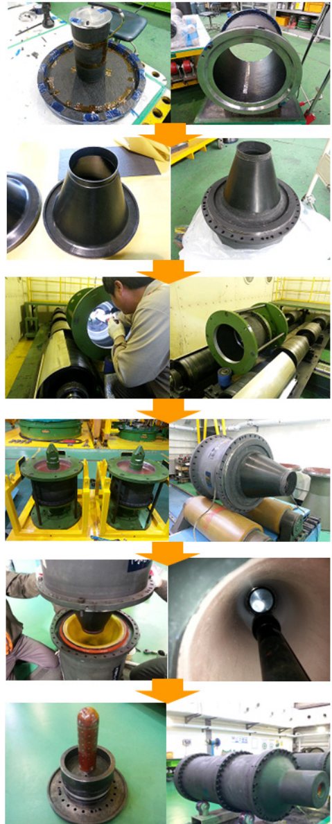
Fig. 6. Fabricating process of dual pulse motor
