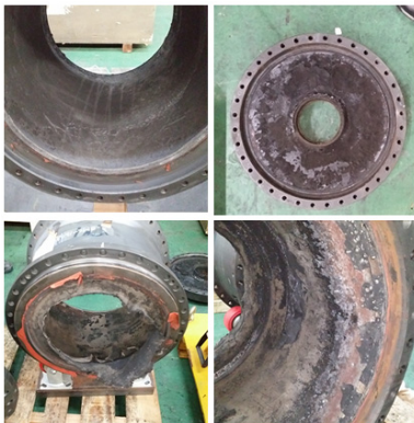
Fig. 22. Ablation of the pulse motor case and PSD after test of 1st/2nd pulse motor(delay time : 60sec)
