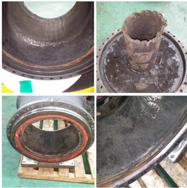
Fig. 21. Ablation of the pulse motor case and PSD after test of 1st/2nd pulse motor(delay time : 2sec)
