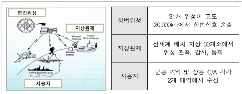
Fig. 2. Basic GPS system
