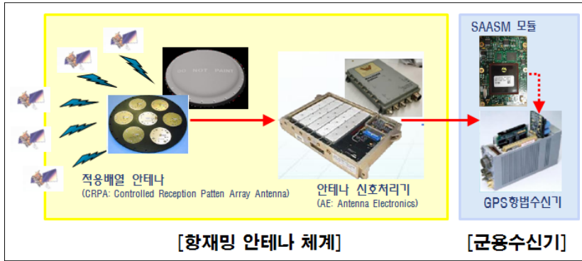
Fig. 3. Composition of anti-jamming GPS system
