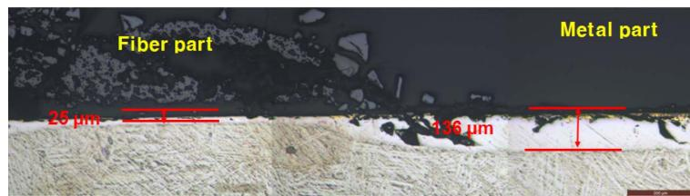
Fig. 17. A photo of an oxide film of a specimen with 4 line thickness SiC<sub>f</sub>/SiC composite protective films manufactured with PCS coating and two times of supercritical carbon dioxide filling after oxidation at 1200°C for 10 min.
