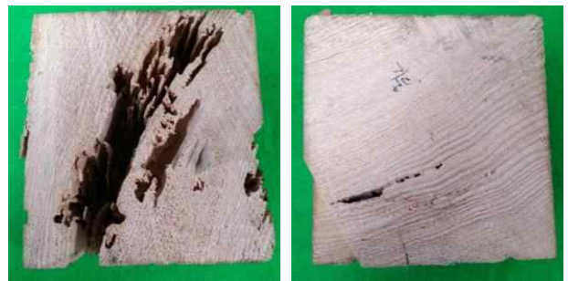
Fig.1 Typical Termites Damages in Dismantled Wood Members of Old Wooden Heritage
