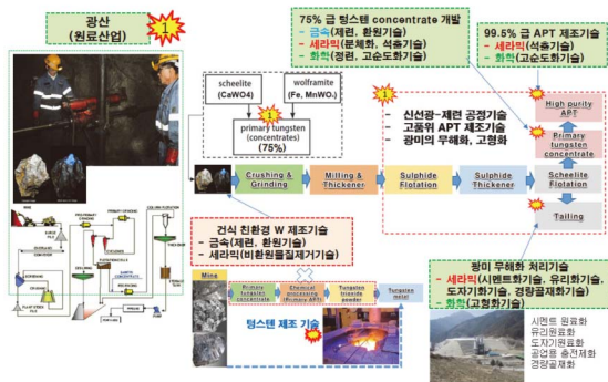
Fig. 9. Tungsten materialization of crude ore with fusion technology.
