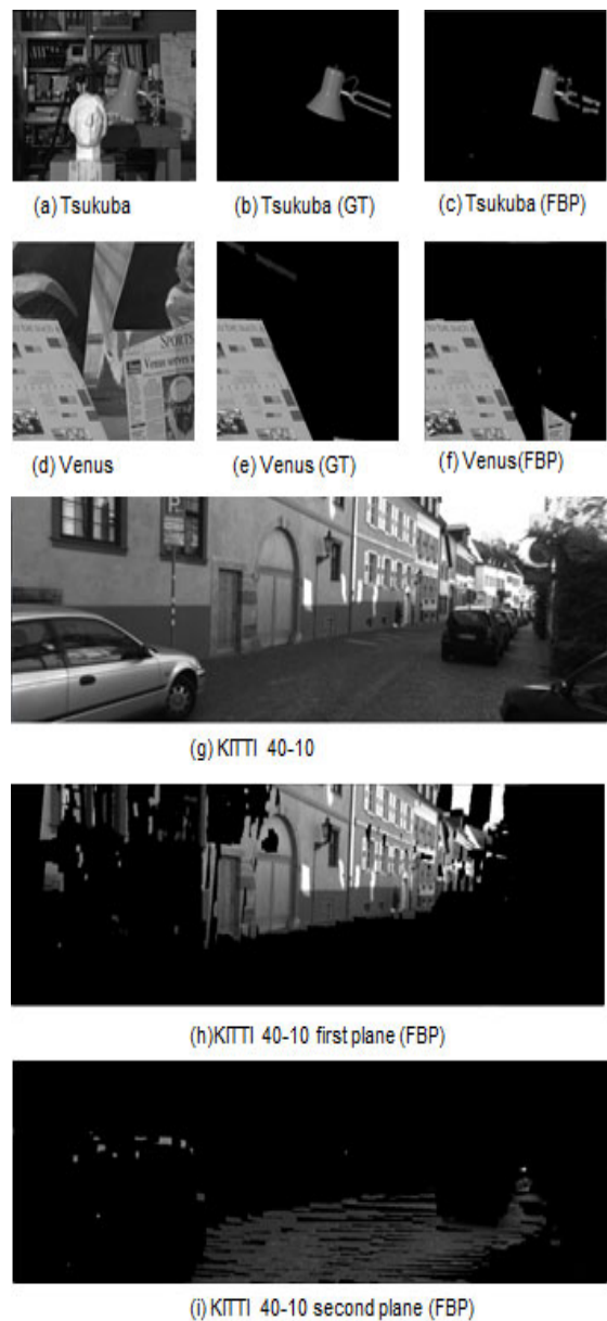
Fig. 7. (a)(d) Original Images in Middlebury Dataset (g) Original Image in KITTI Dataset (b)(c)(e)(f)(h)(i) are Planes Extracted from Ground Truth and FBP Disparity Images
