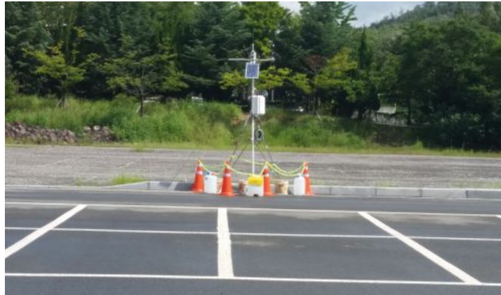
Fig. 1. Automatic weather observation system used in this study installed at a parking lot of Keimyung University.
