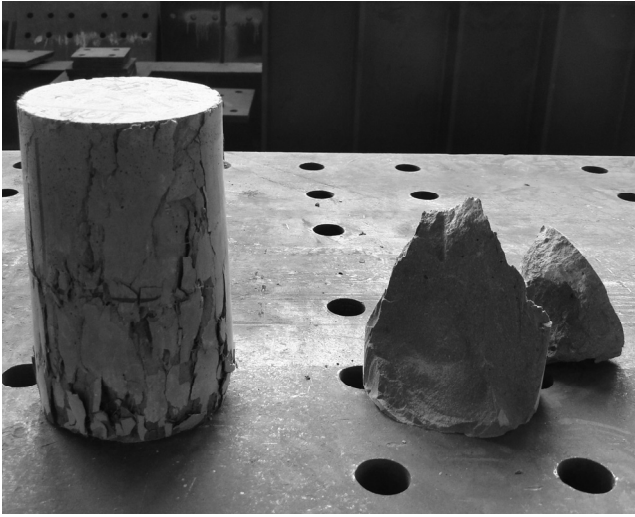
Fig. 3 Failure Pattern of Steel Fiber Reinforced Ultra-High Strength Concrete and Ultra-High Strength Concrete
