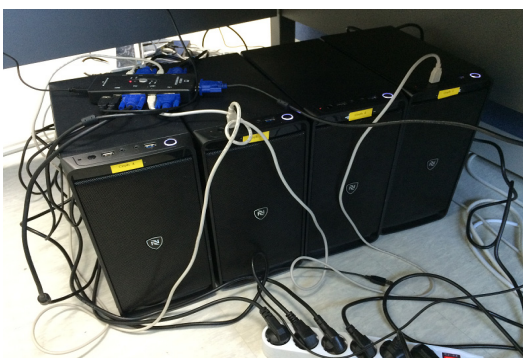
Fig. 7. . Prototype of mass distributed storage system based on PC using Ceph
