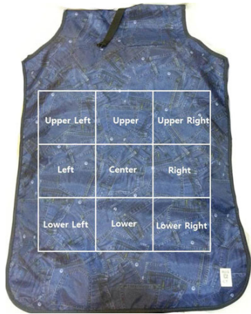
[Fig. 4] Photo of the apron for evaluation of the protection performance. Evaluation areas were divided with the nine sectors: upper left, upper, upper right, left, center, right, lower left, lower, and lower right.
