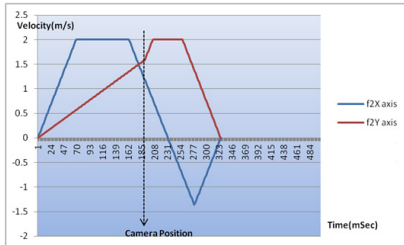
[Fig. 6] Velocity Graph of the Fly2-Motion
