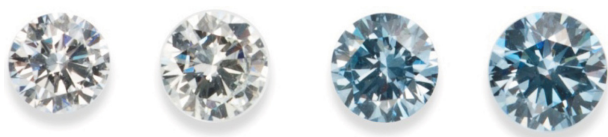
Fig. 1. These polished HPHT synthetic diamond samples (0.25~0.39 ct) obtained from New Diamond Technology (NDT) were examined in this study.
