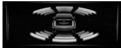
Fig. 4 Front Rear Parking Assist (FRPA)
