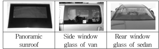
Fig. 8 Use case of ceramic-printed toughened glass
