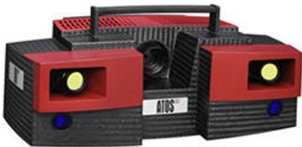
Fig. 2. ATOS III Triple Scan, GOM mbH, Braunschweig, Germany.
