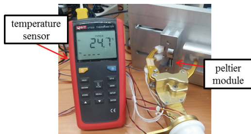
Fig. 8 Experimental setup of sensory feedback system
