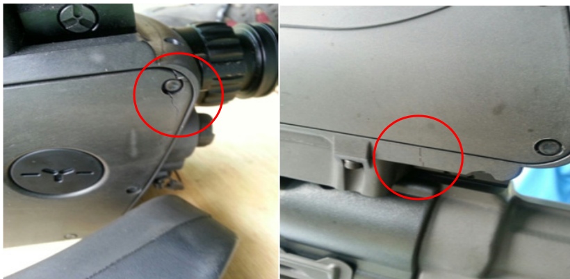
Figure 2. Cracks of K11 Fire Control System
