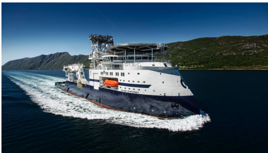
Fig. 10. Drill ship used for directional core drilling at great depth for the Rogfast tunnel
