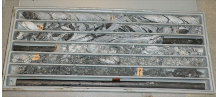
Fig. 9. Example of poor quality rock mass from core drilling at Rogfast (black, thinner sections are tubes representing core loss)
