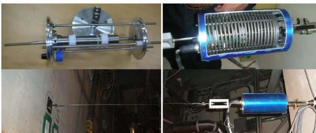
Fig. 1 LVDT and spring assembly, and extensometer mounted on the wall
