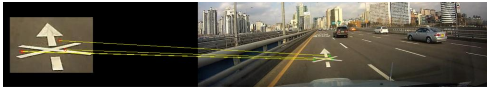
(d) Detection Result of Road Surface Indicators based on SURF Matching
