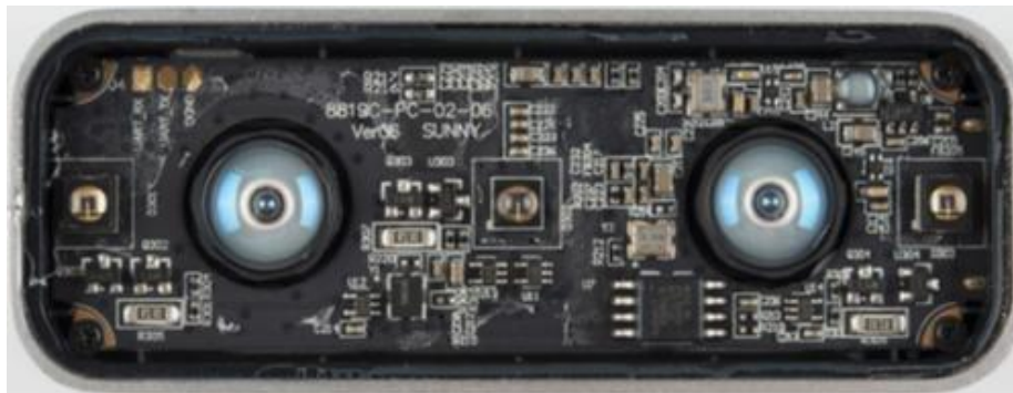
Figure 10. The inside of Leap Motion
