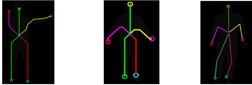
Fig. 5. Body skin joints features representation based on body skeleton model having five joint points using skin color detection technique
