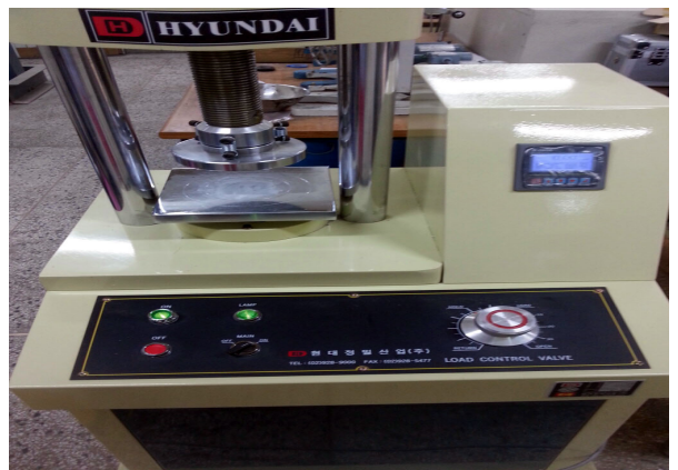
Fig. 2 Compressive Strength Test Equipment
