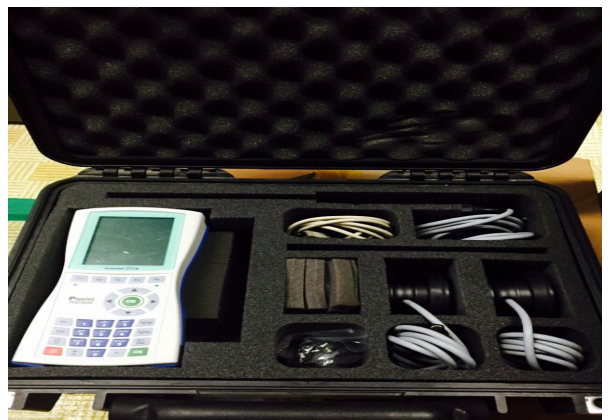
Fig. 3 Thermal Conductive Test Equipment Set, ISOMET-2114
