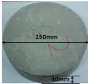
Figure 2. Specimen sample for water absorption test (replacing ratio of BPS = 40%)
