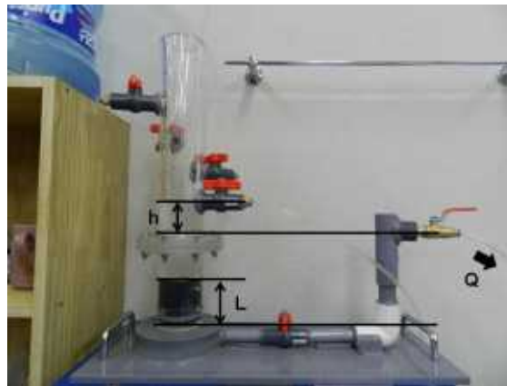
Fig. 2. Constant head permeameter (Lee, 2013)
