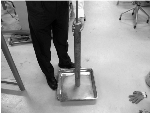
(a) Compaction of specimen
