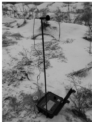
(b) vibrometer and noisemeter
