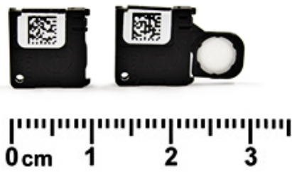
Fig. 3. The OSL nanoDot type used for radiation dosimetry.
