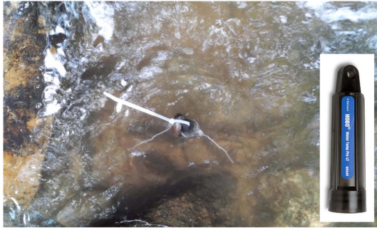
Fig. 2. Photo of the water temperature sensor installation at point 1.
