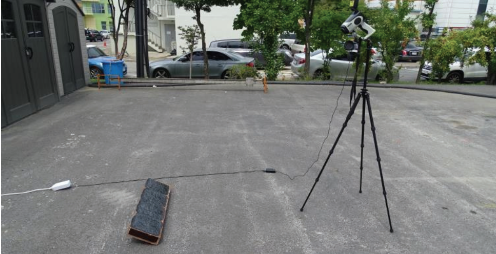
Fig. 4 Thermal imaging techniques applied by using natural light
