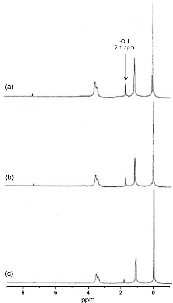
Figure 2. ^1\text{H-NMR} spectra of PUMS depending on reaction time (a) 12 hrs, (b) 18 hrs, and (c) 24 hrs.
