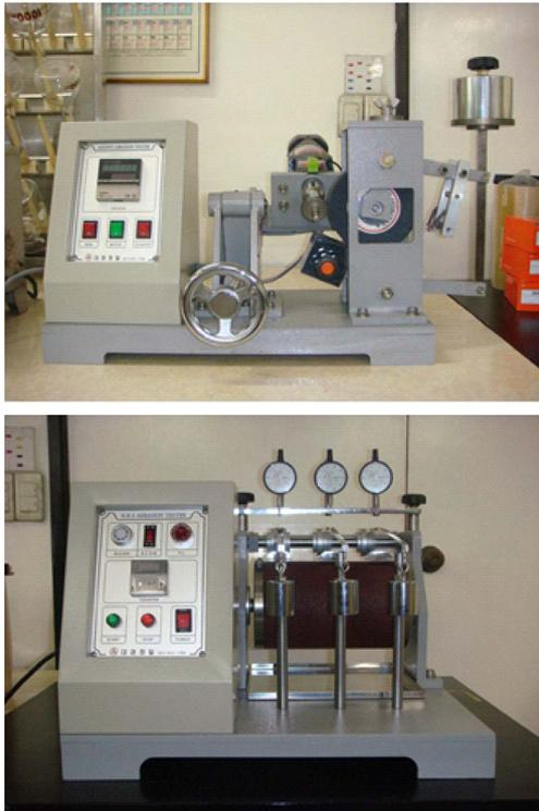
Figure 2. Pictures of Akron & NBS abrasion testers.
