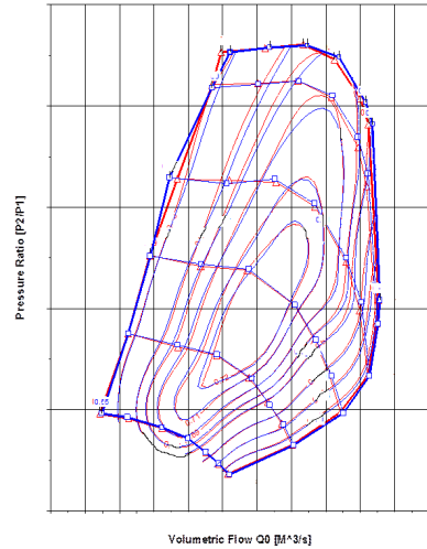
Fig. 14 Compressor performance maps for base (blue) and “Rx=2.0, Ry=0.5 and depth =1.0”(red)
