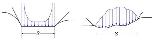
Fig. 1. Definition of complete (left) and incomplete (right) contacts: S designates a contact length.
